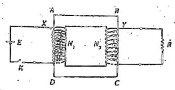
In the diagram shown X and Y are two coils of  $N_1$  and  $N_2$  turns respectively and ABCD is an iron core.
