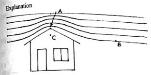
When we consider the streamlines going through the points A and B. As point B is far away, the motion of air is neglegible. By applying Bernoulli's equation for this stream  $P_A + \frac{1}{2} \rho V_A^2 = P_B - 01$ line flow.
