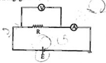
At room temperature of 30°C the voltmeter and ammeter readings are 4.00v and 0.020 A respectively. When the nichrome wire is immersed is an oil bath at temperature 430°C the voltmeter and ammeter readings are 4.05 V and 0.018 A respectively.
