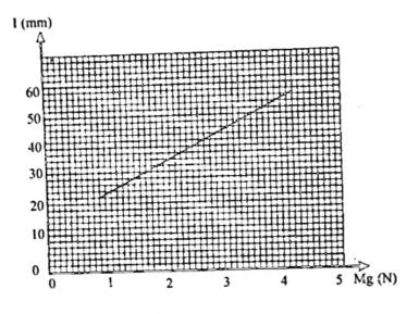
(a) When the block is hung from the spring the length of the spring was found to be 30 mm. Determine the mass of the block, using the above calibration graph.
