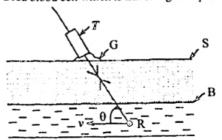
T transmits ultrasound waves with frequency  $f_i$  and after reflection from the blood cell receives them with a frequency  $f_i$   $\theta$  is the ongle between the ultrasound beam and the path of the blood cell.
