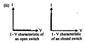
Open switch characteristic resembles that corresponding of cutoff region & closed characteristic resembles that corresponding to saturation region. (or shown on the graphs)
