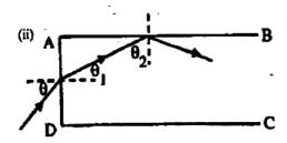
For total internal reflection at AB,  $\theta$ , must be greater than the critrcal angle OR the value obtained in (i)
