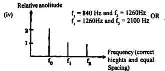
(v) Three electrical Signals having frequencies of, f, and f, and respective relative amplitude 1, 1/2 and 1/2 are superrimposad (mixed)
