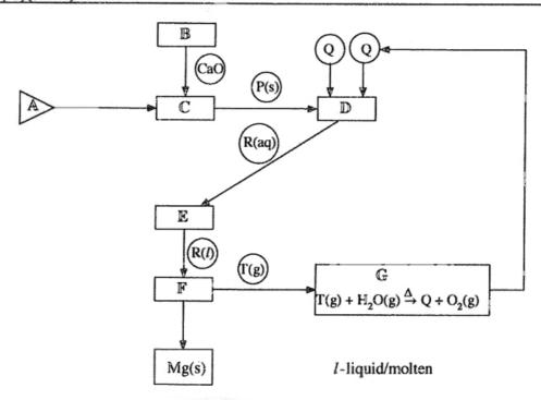
The flow chart given above indicates the production of metal magnesium (Mg) using the Dow Process.
