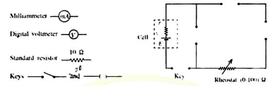
(a) Complete the circuit diagram correctly by drawing the appropriate symbols of the items given above
