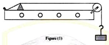
(a) In this experiment the fundamental mode of resonance of the wire is used. What is the reason for this?
