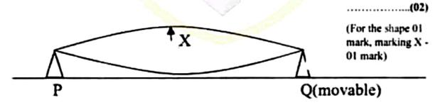
(c) (i) The distance between the bridges in part (b) above is I and the frequency of the tuning fork is f. Write down an expression for the speed (v) of transverse wave in the sonometer wire in terms of I and f.
